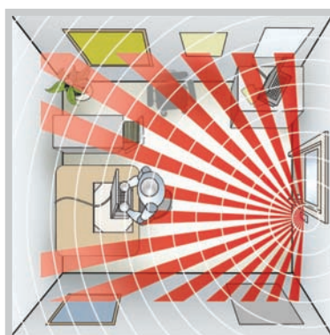
WSD PDT PRIVATE OFFICE WITH OCCUPANT'S BACK TO SENSOR
